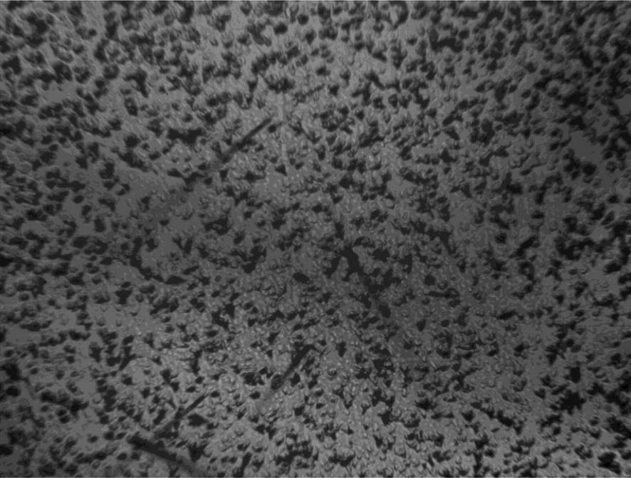
In the field of view of  $284 \times 226 \mu\text{m}$  in olivine; density of tracks,  $1.5 \cdot 10^6 \text{ cm}^{-2}$ .
