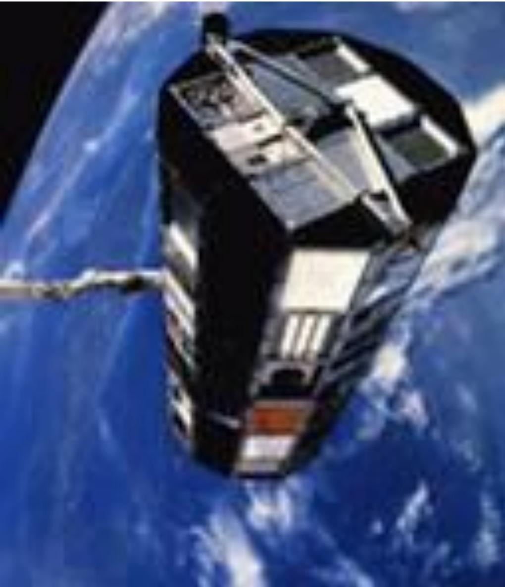
PTD assemblies, also made up of lexan plates, with lead plates located between them (UHCRE — Ultra Heavy Cosmic Ray Experiment experiment) were exposed at an altitude of **450 km for 69 months** on the LDEF space station. In total, about **2500 tracks related to nuclei with  $Z > 65$**  were recorded in this experiment.
