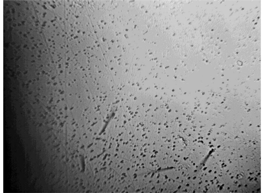
Micrograph of a fragment of olivine crystal surface with a large change of track density. Image size,  $284 \times 226 \mu\text{m}$  the density of tracks within a distance of  $800 \mu\text{m}$  changes by two orders of magnitude, from  $3 \cdot 10^6$  up to  $4 \cdot 10^4 \text{ cm}^{-2}$ .
