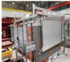
RPC prototypes built and successfully operated for muon flux and charm production measurement at SPS in 2018
